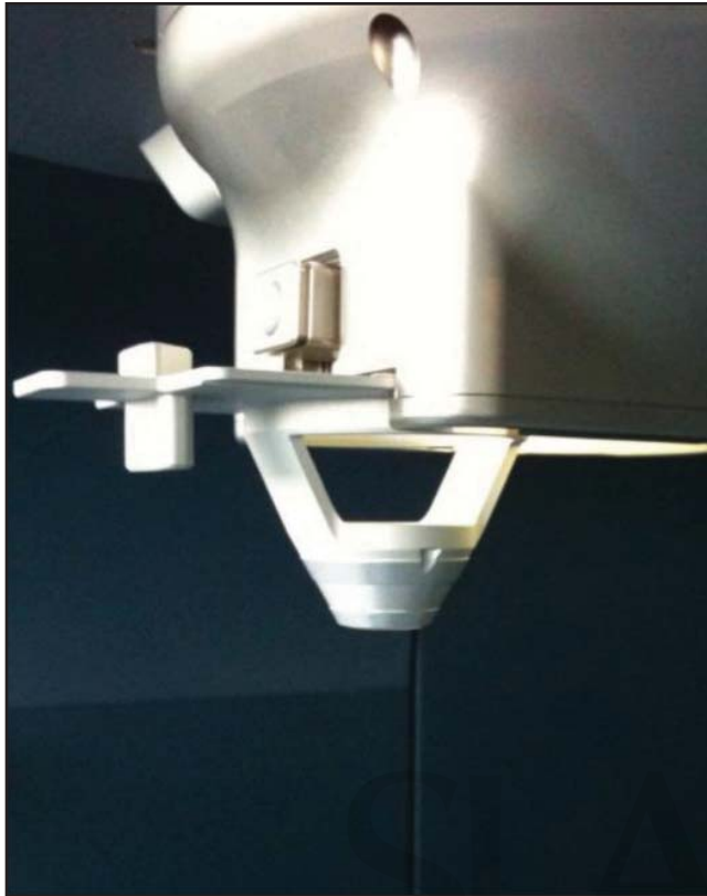
Figure 11-3. The patient-interface cone from the FS200 ready to be inserted into its lock position.
